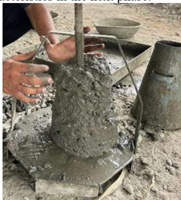
Fig-12: Slump Test
