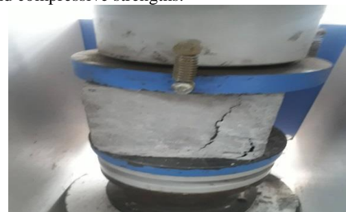
Fig. 3: Compressive strength testing machine
